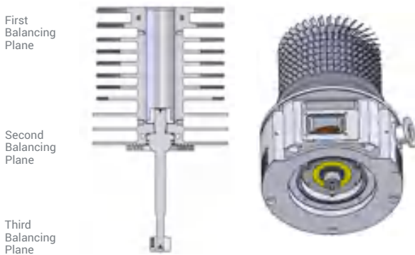
Rotor for Modal Balancing, with three balancing planes
